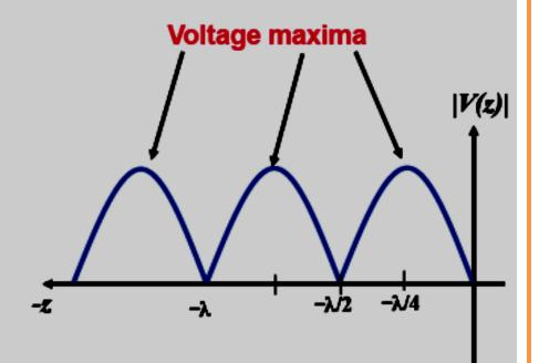
\*Voltage minima occurs at same place that impedance has a minimum on the line
